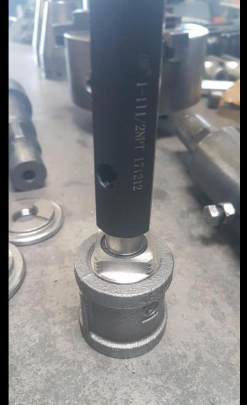
Yellow passivated electrolytic zinc offers corrosion resistance while avoiding the use of chr6+. Instead, we utilize chr3+. This approach guarantees topquality electrical zinc coating without harming the environment.
